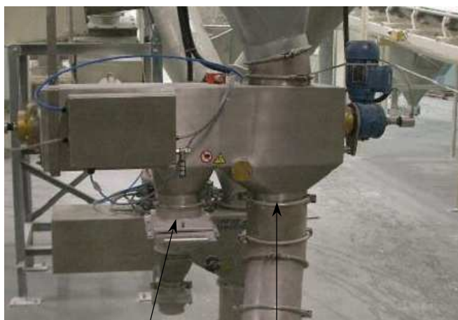
Reject chamber outlet Product outlet
