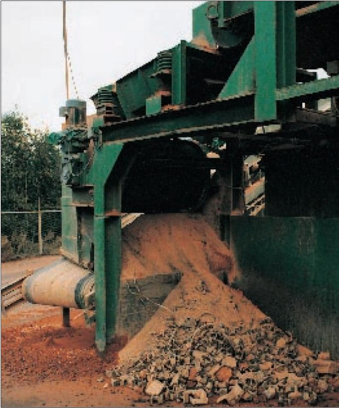
*Drum magnet in use for mineral extraction*
