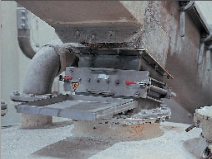
*Bakker Magnetics Magbox ferrous separation system in the feed industry*
