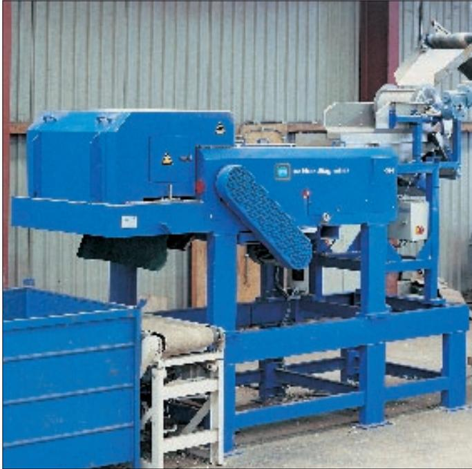
Bakker Magnetics supplies the range of new generation Eddy Current non-ferrous metal separation systems for use in, for example, the waste disposal and recycling industries. Through the introduction of a completely new 18-pole magnet cylinder, the efficiency is greatly improved. In many applications, the separation can almost reach 100%. In recent tests in the glass recycling industry, the efficiency reached 99.8%.
