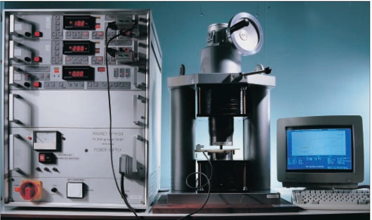
*Permagraph for the analysis of the magnetic properties of material*
