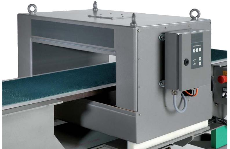
TMDL tunnel metal detectors, which are separable and equipped with digital technology, are used for inspecting bulk materials or individually packaged product on belt conveyors, material slides or vibratory conveyors. They detect all magnetic and non-magnetic metal contaminants (steel, stainless steel, aluminium etc), even those which may be contained in the product. If metal is detected a signal is sent to the process controller or the reject unit is activated.
