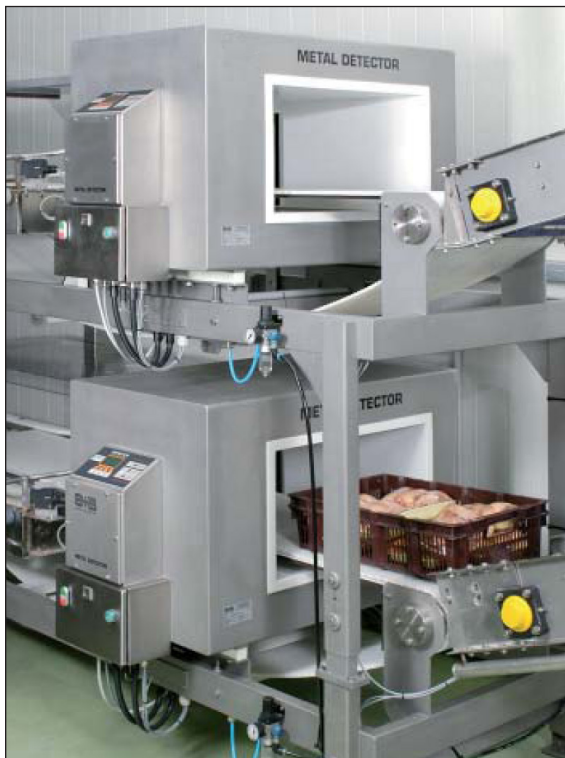
Metal inspection of poultry in E1 containers
