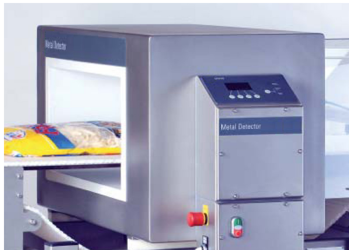
TMD metal detector inspecting potato chips
