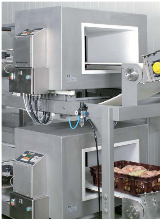
TMD metal detectors integrated in two production lines inspecting poultry products
