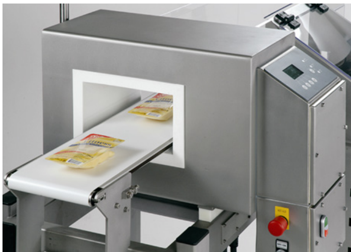
TMD metal detector: final inspection of biscuits
